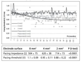
**Conclusions**. Our experience confirms that decreasing tip-electrode surface area has a permanent and significant positive impact on chronic pacing impedance and thresholds.
