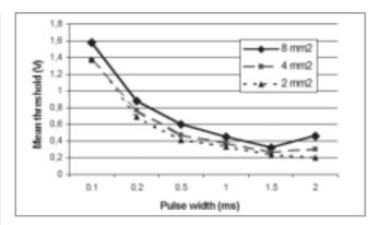
**Conclusions**. Our experience confirms that decreasing tip-electrode surface area has a significant positive impact on acute pacing impedance and thresholds at all pulse width durations.
